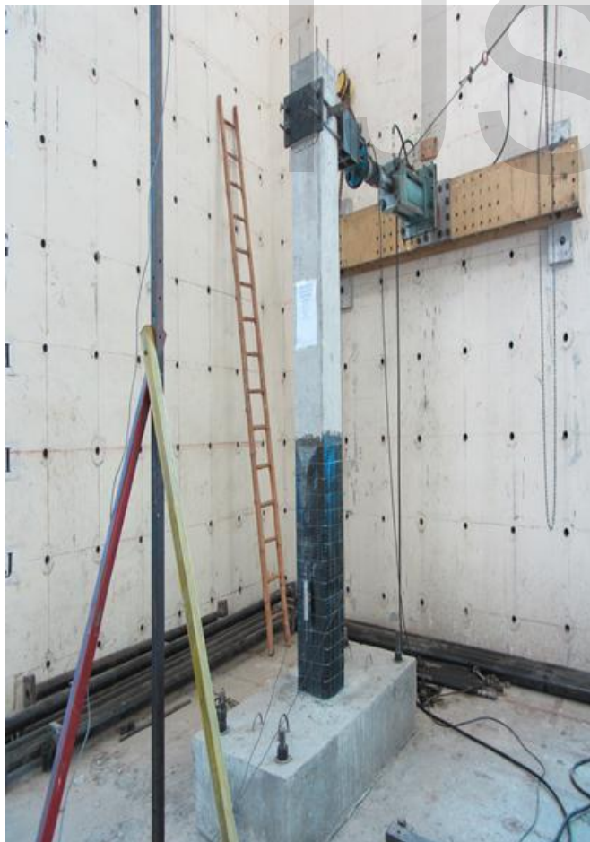
Fig. 5. Testing setup and FRP wrapped section on HF1LC
