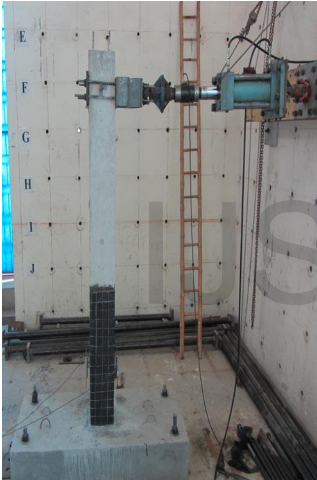
Fig.1. 10-ft full column with testing setup
